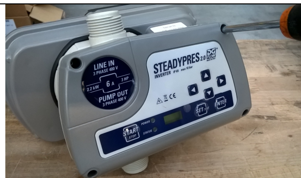
Open the front cover by unscrewing the 4 screws
