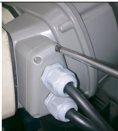
Open the side cover (4 screws)
